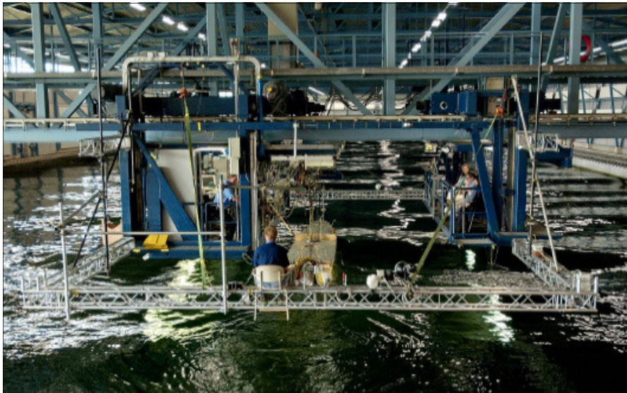
Scale models of the Fast Response Cutter (FRC) and its Rigid Hull Inflatable Boat (RHIB) are tested in the tow tank at the Maritime Research Institute Netherlands (MARIN) earlier this year. Data recorders for the test are located to the left of the towing carriage. The free-sailing FRC model is steered by autopilot. The free-sailing, radio-controlled RHIB model, shown here entering the FRC model's stern ramp, is steered by a trained operator. (Photo Courtesy of Northrop Grumman/MARIN)
