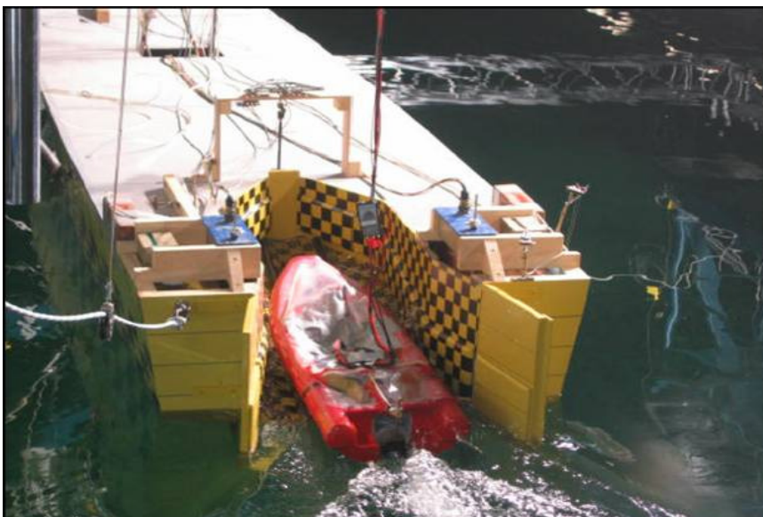
The Fast Response Cutter's design for a stern ramp for small boat launch-and-recovery operations is an area of special interest during tow tank testing. Here, the radio-controlled RHIB model enters the cutter's stern ramp during a test sequence. Realistic model testing in varied wave conditions will lead to continued refinements in the ramp's design. (Photo Courtesy of Northrop Grumman/MARIN)
